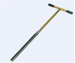
The single gouge auger for soft soils is used for sampling to a depth of 50 cm. The gouge auger supplies undisturbed samples and is suitable for various types of profile research.
