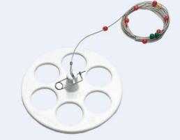
The visibility disc according to Secchi is used to measure water transparency or turbidity in bodies of water. This is a simple device to determine the visibility depth. It is lowered in the water with a wire.
