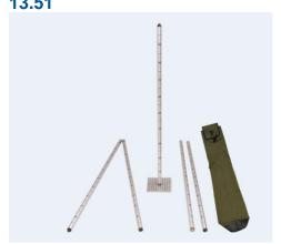
The sediment level stave is part of the standard set to measure the depth of sediment down to a depth of 4 metres. A sediment level stave is a sounding rod used for sounding the sediment layers in surface waters. Either a point or a sediment grid can be mounted to the bottom.
