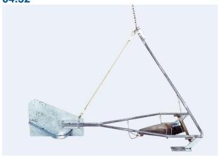
The bed-load transportmeter, type Arnhem is a sampler, used to measure bed-load of coarse sand and fine gravel in rivers and in other watercourses.
