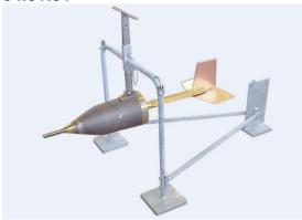
The Delft bottle type suspended load sampler is the standard set for sampling sediment particles larger than 50 µm in rivers and other water courses. This set is applicable in velocities up to 2.5 m/s and can be used at any depth.
