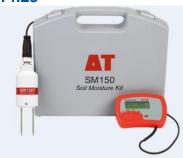
The soil moisture kit is an affordable instrument for obtaining reliable moisture measurements. The HH150 Meter displays volumetric water content (% volume) and is suitable for Horticulture research.
