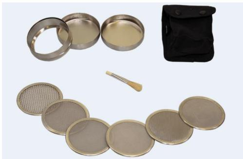
The mini hand sieve set is used to determine the particle size distribution of small quantities of soil. This mini set is pocket-sized and contains several sieve discs: Ø 100 mm, sieve openings: 2.0, 1.0, 0.500, 0.250, 0.125 and 0.063 mm
