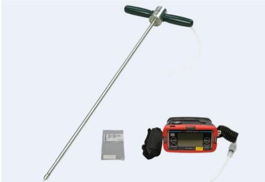
The Soil oxygen content analysis system is a device that helps to carry out a soil gas analysis. Using a 'piercing probe' and an oxygen content meter the growing conditions for shrubs and trees can be defined without time consuming soil drilling.
