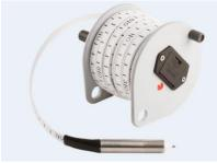
With this water level meter you can take measurements to a depth of 33 feet (10 meters). The pocket water level meter has acoustic and light signals when the probe comes into contact with a conductive liquid.
