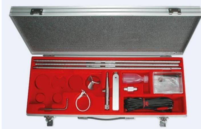
Mini current meter with aluminium propeller of 2 inches (50 mm) in diameter. Used for current velocity determination in small ditches with low water levels.
