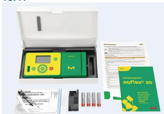
The RQflex Reflectometer is suitable for measuring various anions and cations in soil, water, compost, (pressed) plant material, substrates, etc. The device is portable, for easy use in the field.
