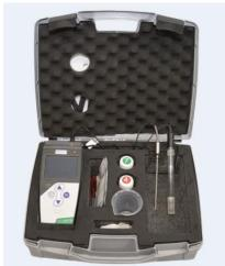
The pH meter for soil and water is a professional portable pH meter with a clear color display. The meter is suitable for measuring in a range of pH between 0-14 pH and a temperature range of 32 to 176 °F (0 to 80 °C).
