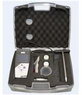
This professional and portable conductivity meter has an innovative high-resolution color display. The Electrical Conductivity (EC) meter is ideal for taking measurements in the field.
