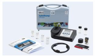
The infrared turbidity meter TB 211 IR is used for measurement by the intensity of the scattered light at an angle of 90 degrees, digital readout. The measuring range of this turbidity meter is 0.01-1100 TE/F or FNU/NTU. The set is supplied in a handy case.
