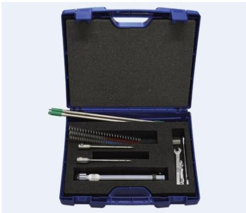
The hand penetrometer for top layers is a device that is used to determine the penetration resistance of top layers. This instrument can also be used for horizontal measurement, for instance in the walls of profile pits, thanks to the limited overall length of the device.
