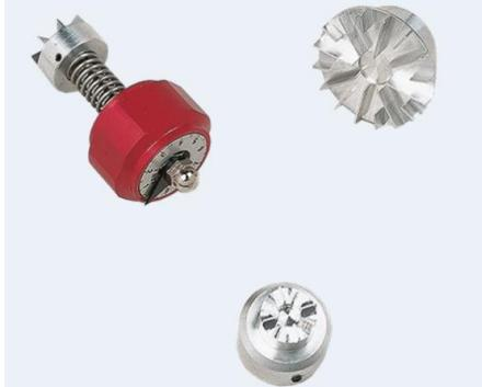
The pocket vane tester is a scientifically designed soil testing instrument for the rapid determination of shear strength of cohesive soils, either in the field or in the laboratory.
