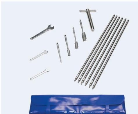
The vane tester can be used to determine the maximum shearing force that can be exercised on a soil. The standard Field inspection Vane tester is suitable for measurements up to 200 kPa (20 t/m<sup>2</sup>).
