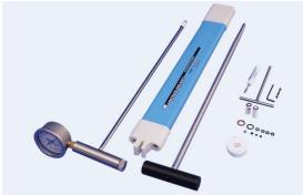
The quick draw tensiometer from Royal Eijkelkamp is a small tensiometer that can easily be moved and, using the auger for pre-drilling, placed into the soil.
