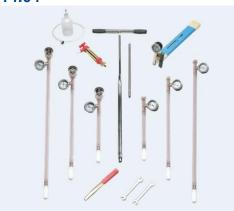
Complete standard set with different types of high quality tensiometers, suitable for multiple measurements. With this set you can do measurements up to a depth of 3 feet (90 centimeter).
