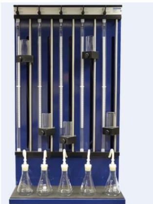
The calcimeter measures the amount of calcium carbonate, or lime contents, in the soil. This is an important indication of the quality of the soil. Measure the carbonate content of a soil sample with the Royal Eijkelkamp calcimeter, created for the simultaneous research of 5 samples according to NEN-ISO 10693. Complete with Erlenmeyer flasks (10 pieces) and test tubes (160 pieces)
