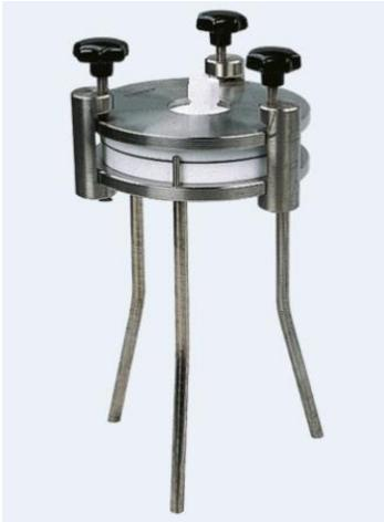
The filter holder for in-line filtration is used for removal of soil particles from water samples during sampling. This apparatus has a net filtration area of 130 cm<sup>2</sup>, and it is suitable for use in the field and in the laboratory.
