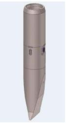
The Royal Eijkelkamp Injection Lance is fitted with a chisel type cone in which a spring retained large valve is mounted. The valve is kept closed by a spring and by the pressure of the groundwater surrounding the chisel. The valve will only open when pressure is applied larger than the pressure of spring, groundwater and (liquefied) soil together.
