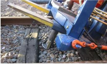
Royal Eijkelkamp has developed a state-of-the-art drilling system to extract core samples from the coarse granite from railway beds and the soil below. There is a need to know more about this material. Higher train speeds, heavier loads and a growing interest in the dangers of pollution, make sampling necessary.
